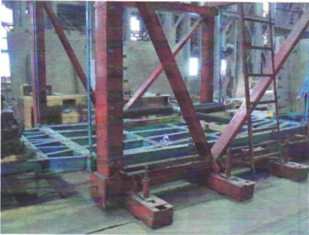
Fig. 6.1. The general view of vibroplatform with the prototype model, laid down on it
